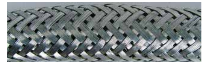
CF27-40-10-02-01-D: After more than 10 million bending movements, no shield wire breakages
