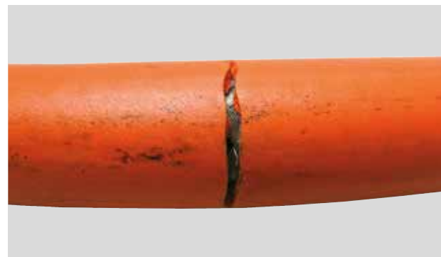
Cracks in the outer sheathing of materials from competitors caused by the "use of oil" in E-Chains®.
