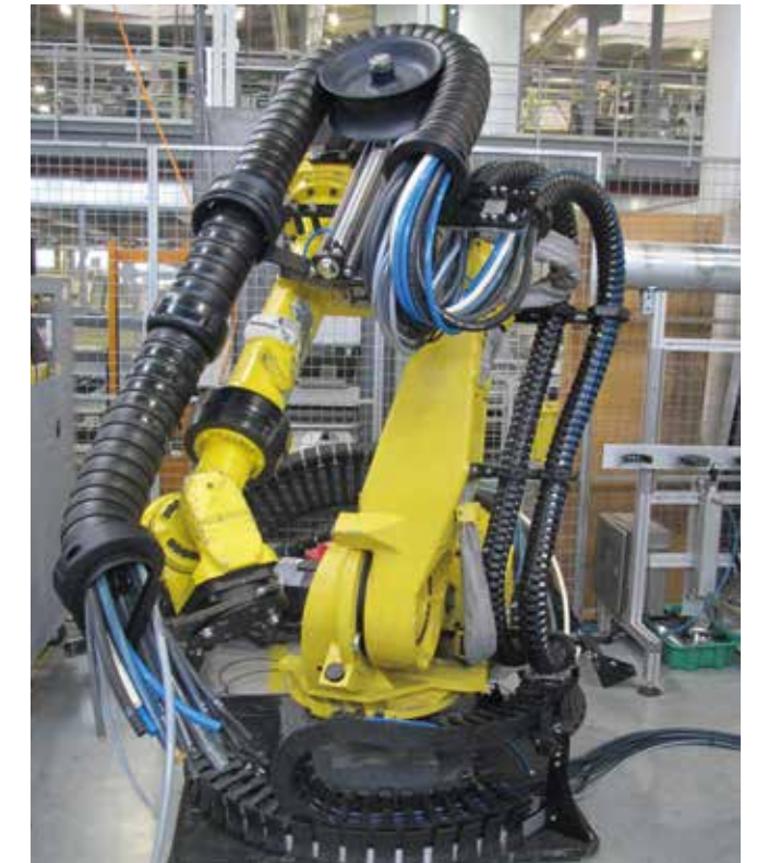
Test for combined motions: simulation of complex motions in robot applications
