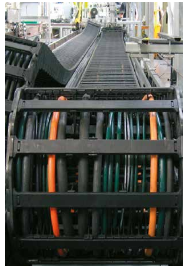
Deliberately non-conforming chain filling in order to simulate a real application.
