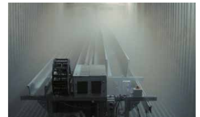
Cold tests on cables and Energy Chains® at -40°F
