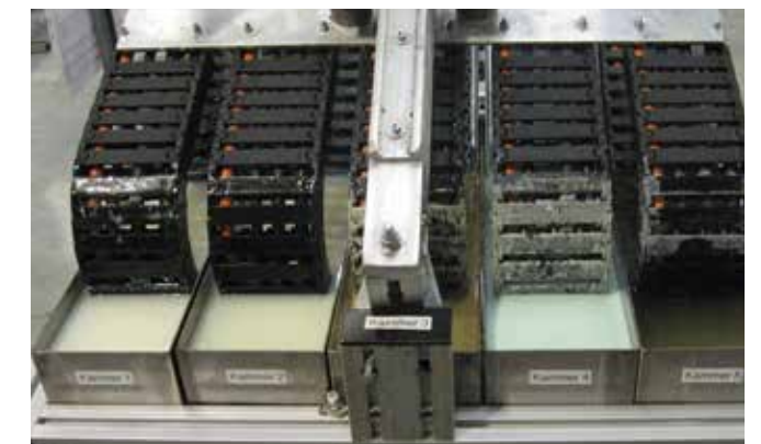
Media test: test of the durability in adverse chemical effects in motion
