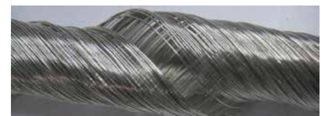
Picture 3: Detail pictures of the CFROBOT after more than 3.0 million movements of \pm 270^\circ
