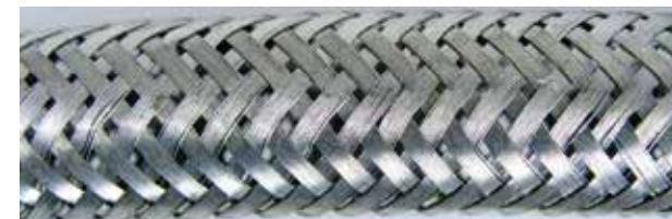
CF21-40-10-02-01-UL: After more than 10 million bending movements, no shield wire breakages
