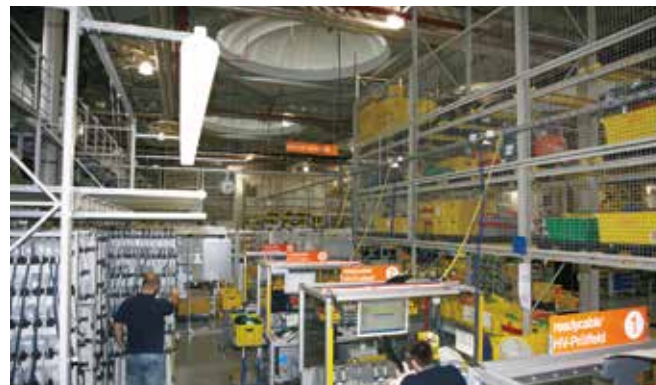
Computer-based high-voltage testing and inspection of all assembled cables
