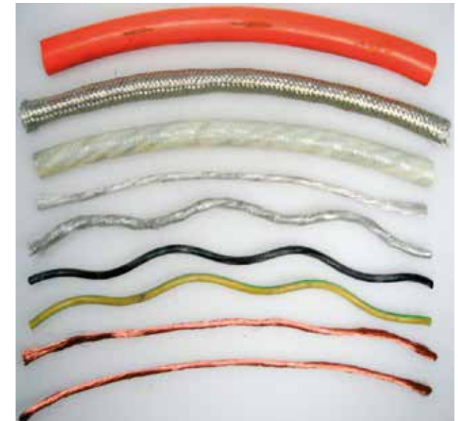
CF27-D: Overall stranding including the outer jacket without damage
