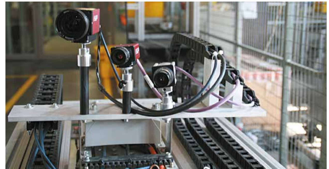
More than 6 million movements in E-Chains® with 32.81 ft (10 m) cable length already successfully tested with FireWire CFBUS-055.
