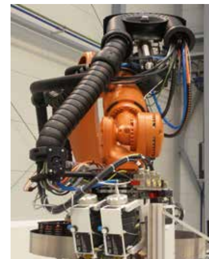
igus® Chainflex® cables in application of a multi-dimensional moving energy chain triflex® R for 6-axis robots.
