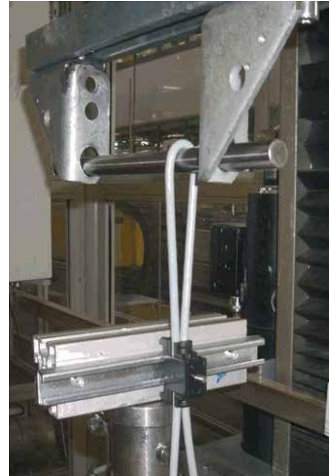
igus® tensile strength test with CFX clamps
