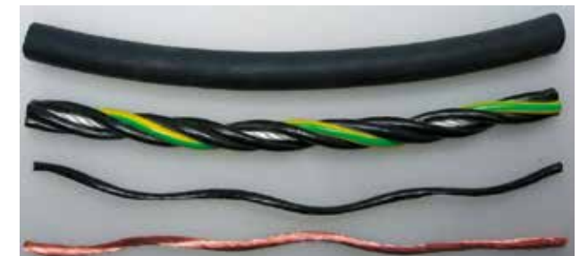
The individual elements of the CF9 from the cable piece dissected for the test setup.
