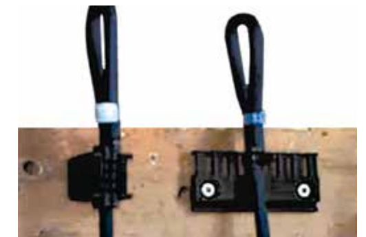
Tensile strength tests with Chainflex® cables
