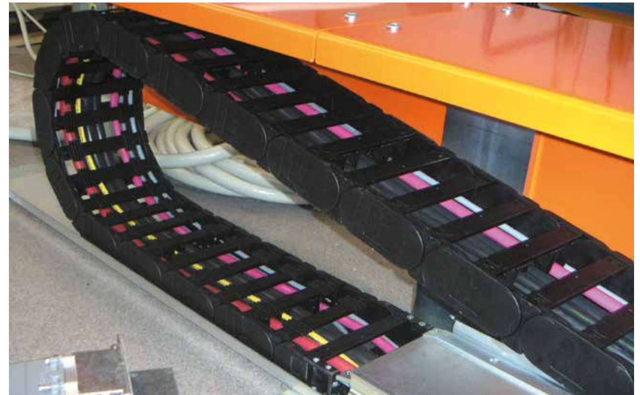
Chainflex® CF2 cables are resistant to oil and coolants. E-chain®: System E4/00
