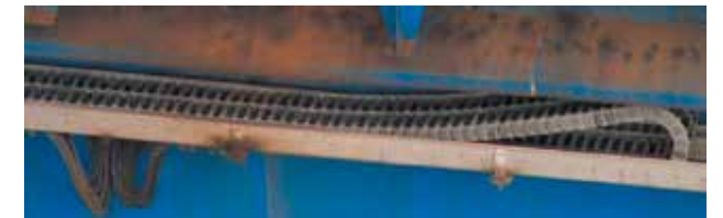
An igus® energy supply system with an approx. length of 85 ft. in a stainless steel trough.
