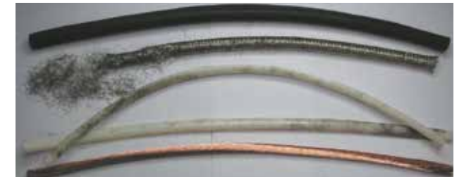
Picture 1: Damaged overall shield sample of the braid version after 250,000 torsional movements
