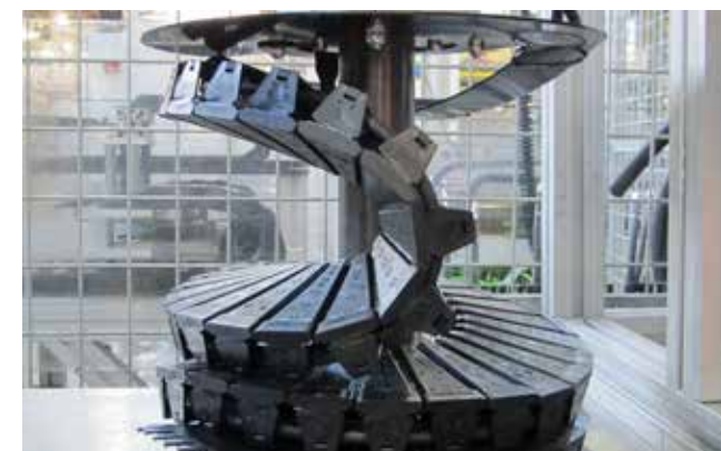
Rotary movement tests: Demanding chain applications with small radii
